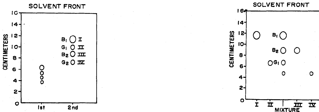
Fig. 1. Separation of aflatoxins on Silica Gel HR plus G-HR (1:1, w/w) after one and two developments with solvent "A".
